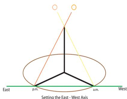
Figure 3: Establishing the exact East-West line (Plofker, 2009)
