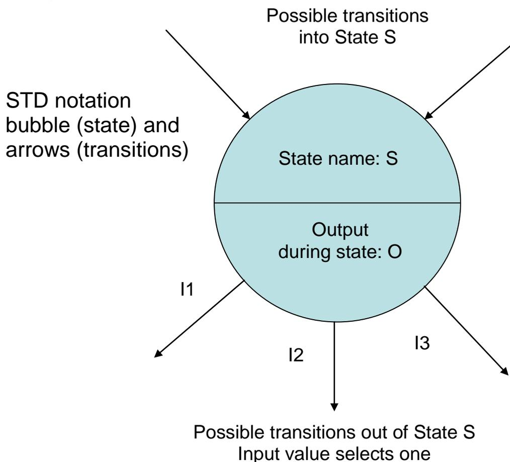
Figure 2. STD notation: a state bubble- containing the State name and Outputs during that state- and possible Transitions in and out of that state with the Input values that select them.
