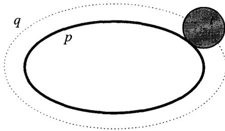
A CNC programmer, for example, was faced with the task of cutting an elliptic shape (denoted by  $p$  in picture on the left) with a milling machine. To accomplish this task he had to calculate the path ( $q$ ) along which the centre of the cutting tool (represented as a circle  $t$ ) should move while cutting the elliptic shape  $p$ . The technician claimed that the offset curve  $q$
