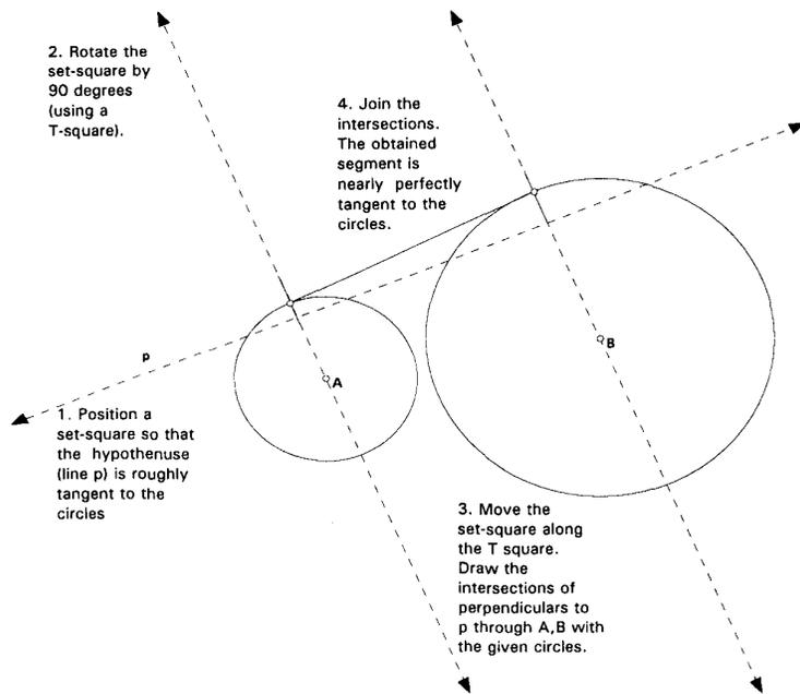
In considering the draftsman's act of joining two circular arcs with segments - as in many examples
