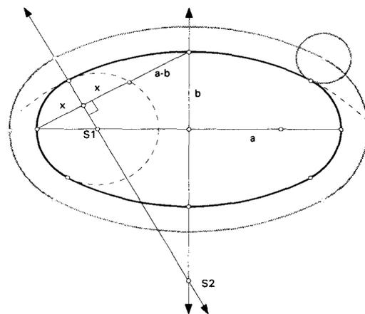
*approximating* an ellipse with four circular arcs. The construction is shown on picture above.)
